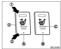
The front seats are warmed by built-in heaters. The switches located on the center console can be operated independently (driver's side seat (A) and front passenger's side seat (B)) of each other.
