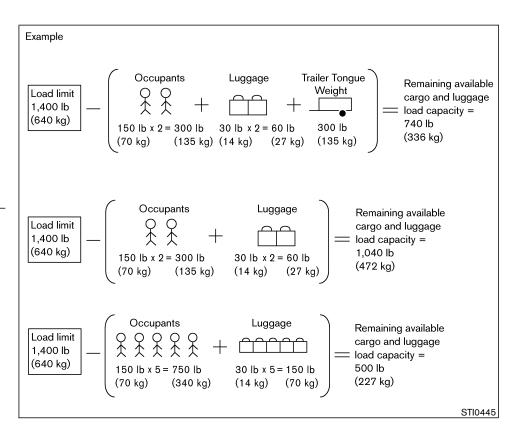
Steps for determining correct load limit
