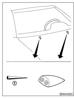
If you wax the surface of the hood, be careful not to let wax get into the washer nozzle. This may cause clogging or improper windshield washer operation. If wax gets into the nozzle, remove it with a needle or small pin (1).
