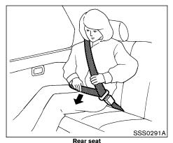
If the seat belt cannot be pulled from its fully retracted position, firmly pull the belt and release it. Then smoothly pull
