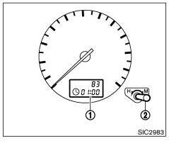
Turn the adjusting knob left to adjust the hour. Turn the adjusting knob right to adjust the minutes.
