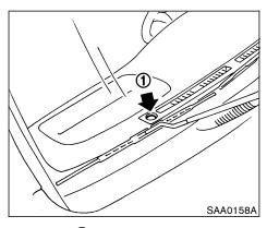
The sensor (1) on the instrument panel helps maintain a constant temperature; do not put anything on or around this sensor.
