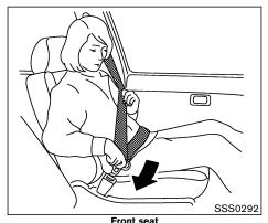
THREE-POINT TYPE SEAT BELT WITH RETRACTOR
