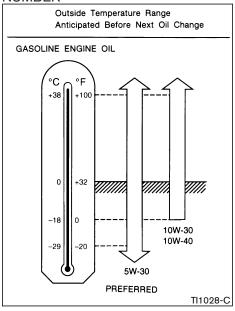
SAE 5W-30 viscosity oil is preferred for all ambient temperatures. SAE 10W-30, 10W-40 viscosity oil may be used if the ambient temperature is above -18°C (0°F).
