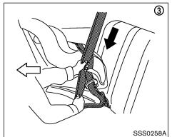
3. Pull on the shoulder belt until all of the belt is fully extended. At this time, the belt retractor is in the automatic locking mode (child restraint mode). It reverts back to emergency locking mode when the belt is fully retracted.
