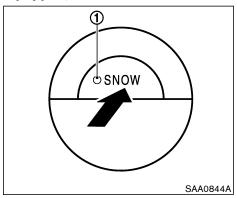
For driving or starting the vehicle on snowy roads or slippery areas, push the SNOW mode switch and indicator light (1) on the switch will illuminate. When the SNOW mode is activated, engine output is controlled to avoid wheel spin.
