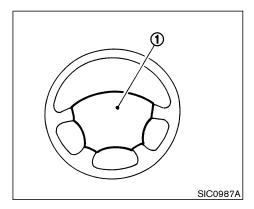
To sound the horn, push the center pad area (1) of the steering wheel.
