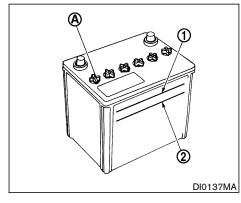
Check the fluid level in each cell. It should be between the UPPER LEVEL (1) and LOWER LEVEL (2) lines.
