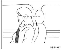
Adjust the head restraints so the center is level with the center of your ears.
