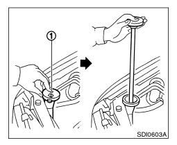
The low washer fluid warning light comes on when the washer tank fluid is at a low level. To check the fluid level, use your finger to plug the center hole 1 of the cap/tube assembly (as shown above), then remove it from the tank. If there is no fluid in the tube, add fluid. Add a washer solvent to the water for better cleaning. In the winter season, add a windshield washer antifreeze. Follow the manufacturer's instructions for the mixture ratio.
