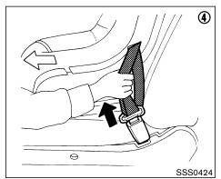
Allow the belt to retract. Pull up on the belt to remove any slack in the belt.
