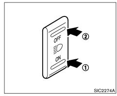
To turn the driving light on, push the "ON" side (1) of the driving light switch when the headlight switch is in the (high beam) position.
