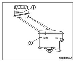
For additional fluid specification information, refer to "Capacities and recommended fuel/lubricants" in the "9. Technical and consumer information" section.
