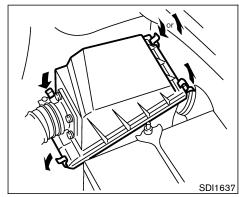
The filter element should not be cleaned and reused. Replace it according to the maintenance log shown in the separate Service and Maintenance Guide. When replacing the filter, wipe the inside of the air cleaner housing and the cover with a damp cloth.
