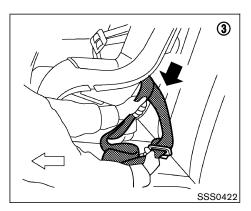
Pull on the shoulder belt until all of the belt is fully extended. At this time, the belt retractor is in the automatic locking mode (child restraint mode). It reverts back to emergency locking mode when the belt is fully retracted.
