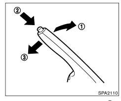
**To apply:** pull the parking brake lever up ①.
