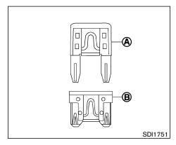
Some vehicles are equipped with engine compartment and passenger compartment fuse boxes that use only type (A) fuses. Other vehicles are equipped with type (A) fuses in the engine compartment fuse box and type (B) fuses in the passenger compartment fuse box.
