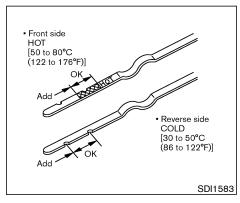
If the vehicle has been driven for a long time at high speeds, or in city traffic in hot weather, or if it is being used to pull a trailer, the fluid level cannot be read accurately. You should wait until the fluid has cooled down (about 30 minutes).
