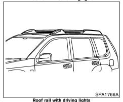
Luggage can be carried on the roof by securing crossbars to the roof rails. Follow all crossbar manufacturers instructions for installing and use of the crossbars. The roof rails are designed to carry loads (luggage plus crossbars) below 100 kg (221 lb). Overloading may cause damage to the vehicle.
