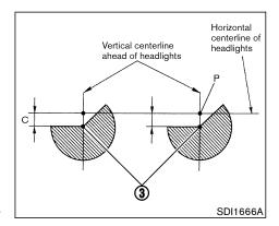
Be sure that the vehicle is parked directly vertical to the wall on which the headlights will be projected.
