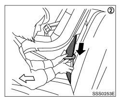
2. Route the seat belt tongue through the child restraint and insert it into the buckle until you hear and feel the latch engage.
